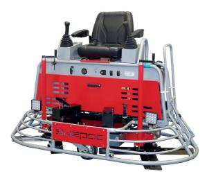
Semi-hydraulic ride-on trowel with joystick control for larger surfaces, intended for levelling and troweling of freshly laid concrete floors.
